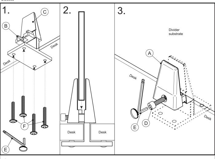
1. Using the relevant screws "F", Fasten part "B" to the desk using tool "E".
