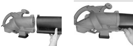
2) Insert lower tube into upper tube and push them until they are connected firmly together then tighten the screws.
